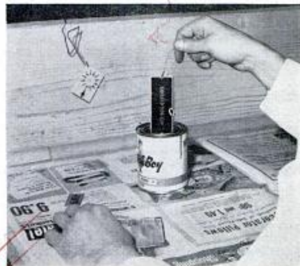
Above, a sharp-pointed knife is used to cut out or scribe lettering before etching. Below, the completed name plate, with enamel baked around the lettering, is dipped in clear lacquer to preserve polish
